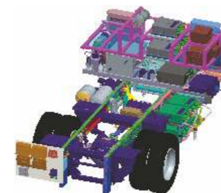
The fuel stack is fitted on the rear module of the bus, as shown below:
